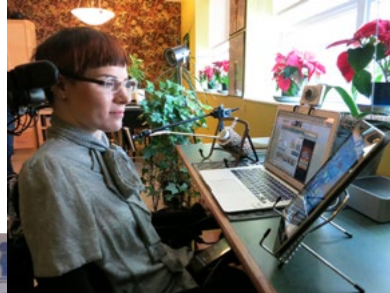
Carolyn Piro works at her computer using voice recognition software and an optical head mouse. (Photo: UHN)
